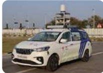
Safari (Data Collection Vehicle) by TIHAN. First in India to capture multisensory (LiDAR, RADAR & Camera) data across diverse Indian scenarios, traversed 8,000 km+ from IIT Hyderabad to Jammu to develop autonomous navigation datasets,
